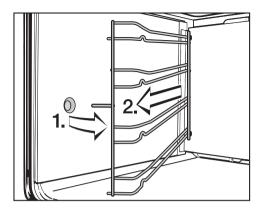
Pull the rails out of holder (1) at the front of the oven and then pull them out of the oven (2).
